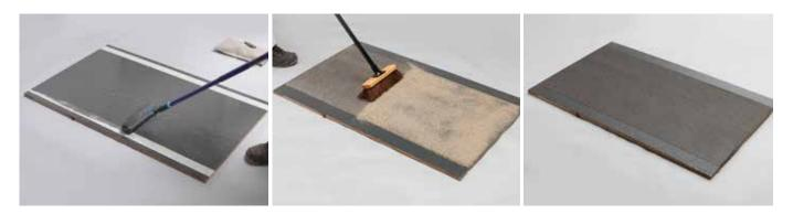
Under BS 7976-2:2002+A1:2013's Pendulum Test assessment of slip resistance, FLS Liquid waterproofing combined with a quartz or granite aggregate achieved an overall classification of Low Slip Potential, or a slip risk of  $\geq$  1 in 1,000,000 users.
