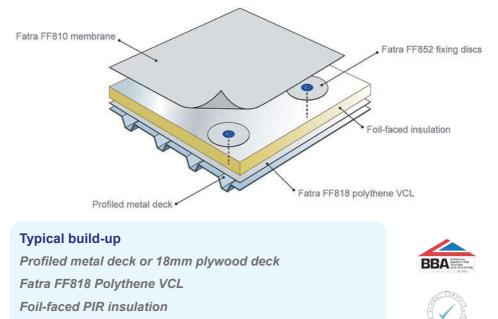
FR-45 Tube washer, FBS-5.8 fixings and FF852 fixing discs
