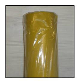
Fatrafol Polyethylene Vapour Control Layers should be installed on the 'warm' side of the insulated structure, with special care being taken to ensure that all seams and holes are sealed effectively - thus rendering the whole structure moisture vapour proof and improving thermal performance. It is important that Fatrafol Polyethylene Vapour Control Layers should be continuous in order to prevent vapour entering the wall or the roof.
