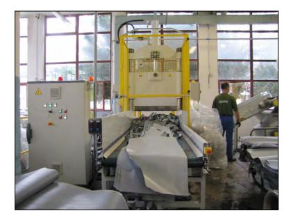
Our factory in the Czech Republic has also invested €30M in a factory based recycling plant. Recent advances have meant that Fatra are now able to include up to 50% recyclate in new roofing membranes.
